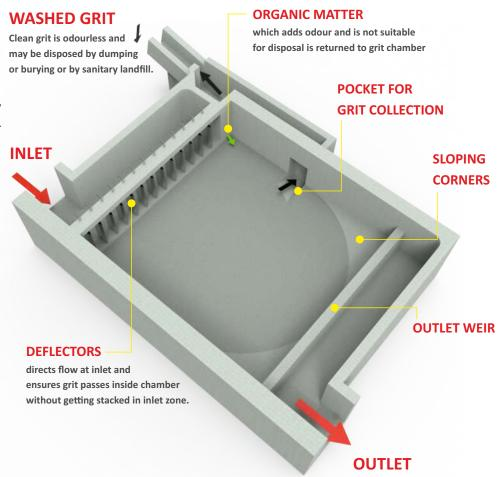
Continuous, mechanically operated grit chamber. Consists of rotating grit collecting mechanisms and a reciprocating rake washing mechanism. Capable of removing 95% of all plus 100 mesh grit at 2.65 specific gravity. Produces a substantially grit-free liquid and cleaned well-washed drained grit.
