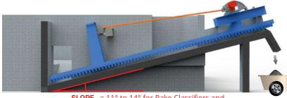
**SLOPE** = 11° to 14° for Rake Classifiers and = 15° to 25° for Screw Classifiers
